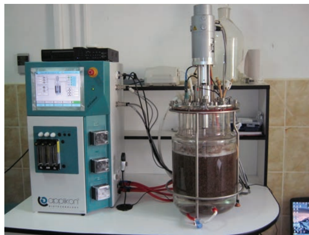
Figure 1. The laboratory-scale bioreactor for submerged cultivation of microbial cells.
