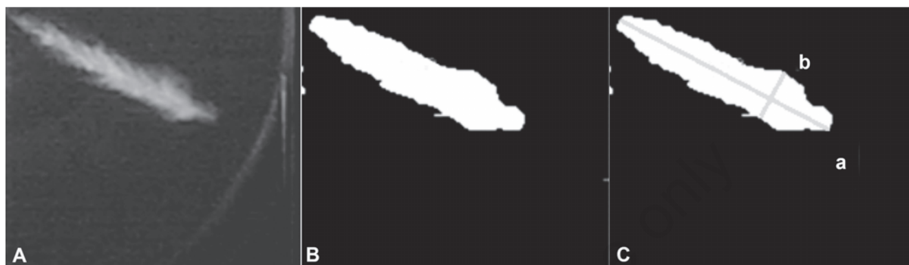
Figure 2. Post-processing phases of the spray images for the estimation of the spray penetration and shape ratio. A) original image; B) image conversion in black and white; C) 'a' is the length of the segment joining the spray tip to its nozzle exit, while 'b' is the highest spray depth in a direction orthogonal to the segment joining 'a' with the spray exit; 'a' is the spray penetration, while 'a/b' is the shape ratio.
