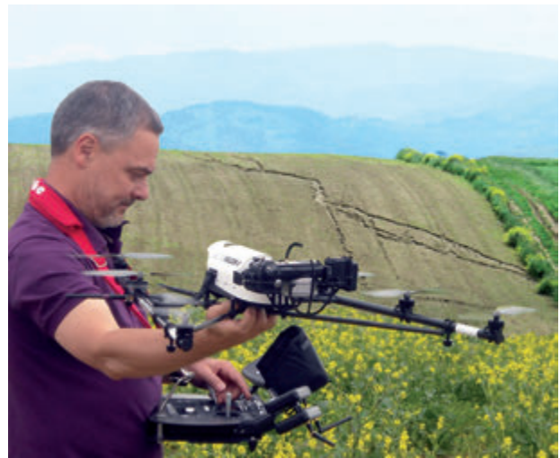
Figure 1. Falcon 8 Octocopter, and remote control station. In the background, a field rilled by soil erosion in one of the study areas of the MO.NA.CO. project.
