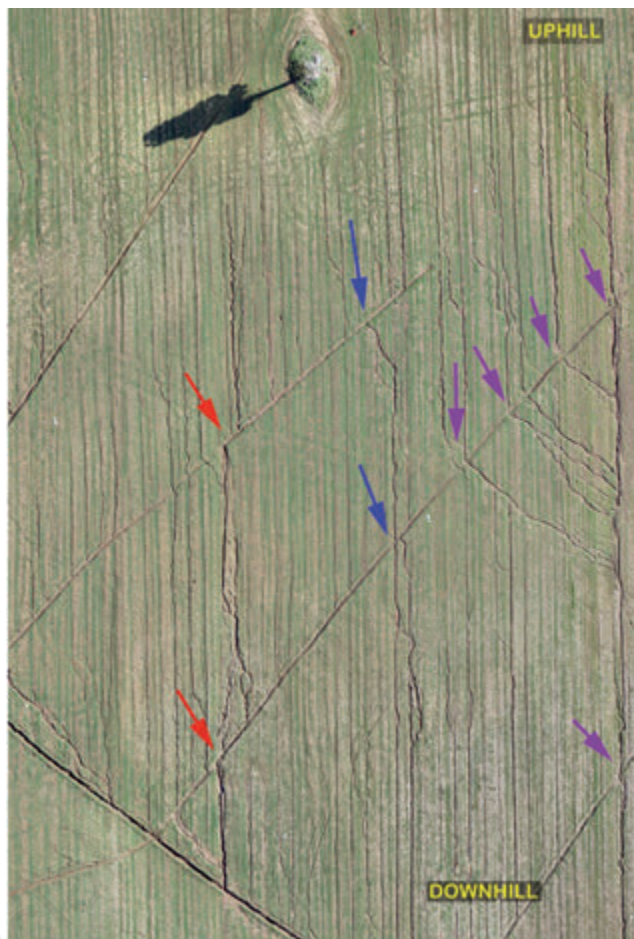
Figure 11. Zenithal picture from drone that illustrates the zones of breakage of the temporary ditches because of their undersize. Arrows of different colours identify different rills and indicate points where runoff has not been effectively intercepted by ditches, causing a 'domino effect' of concentration of erosion downstream (Tor Mancina farm).
