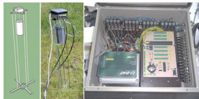
Figure 1. Automatic soil respiration system. Left, schematic view of automatic chamber design. Middle, automatic chamber installed on the field. Right, central data storage electronic with multiplexer containing 2x16 electromagnetic valves.
