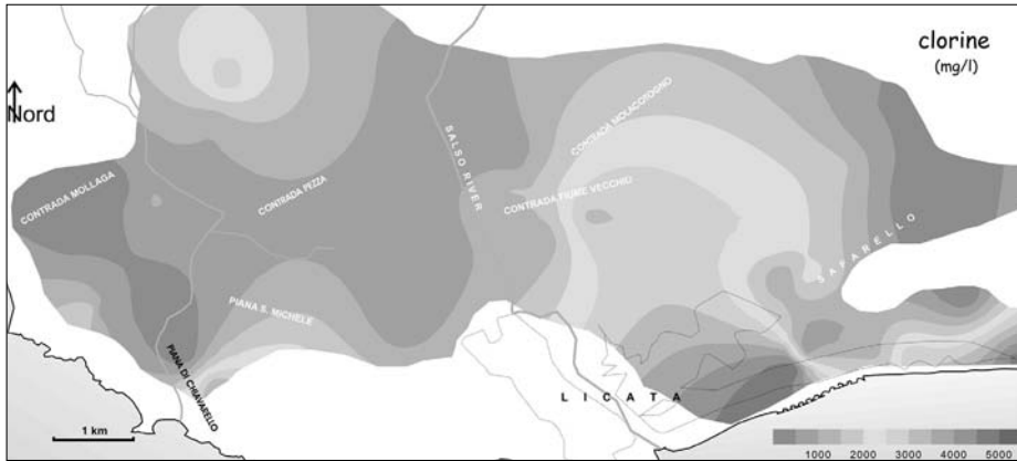
Figure 12. Space distribution of the chloride concentration (mg/l; for the location of the monitored wells see Fig. 9).
