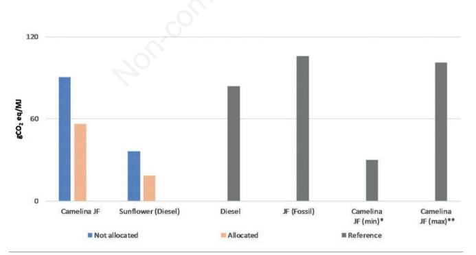
Figure 2. Comparison of camelina Jetfuel (JF) GHG with different propellants (\*Li and Mupondwa, 2014; \*\*Lokesh et al., 2015).
