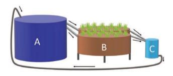
Figure 1. Experimental unit layout. A: tank for fish in aquaponic treatments or nutrient solution for hydroponic treatments (500 L); B: tank for vegetables/biofilter (275 L); C: storage tank for water (50 L). Arrows indicate water flow direction.
