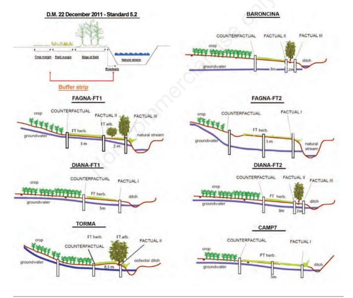
Figure 1. Experimental schemes of the experimental sites and their comparison with the general case contained in M.D. 27417.
