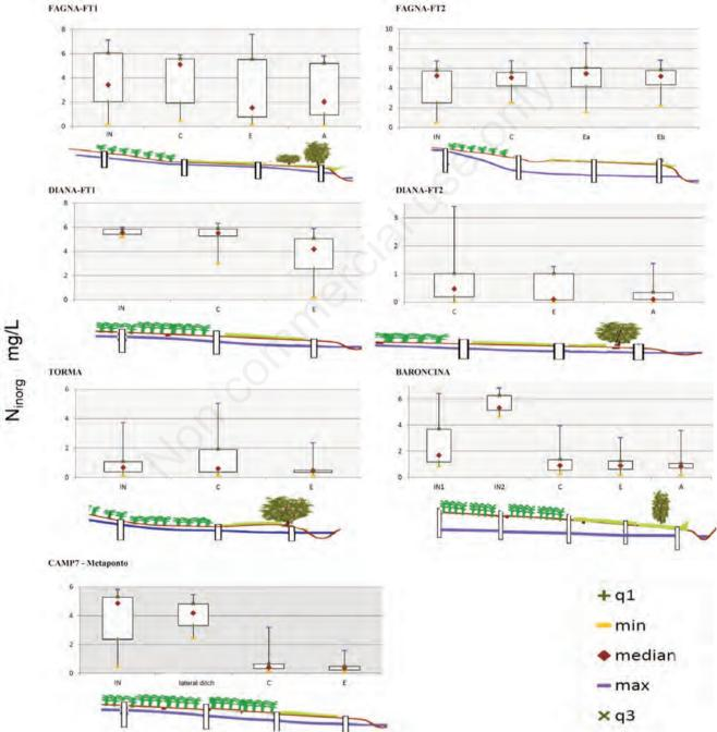
Figure 4. Comparison between the concentration values of dissolved inorganic nitrogen in different points of the monitored systems.
