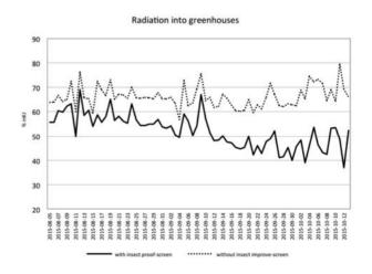
Figure 15. Difference in transmitted radiation between external and internal environment in the different greenhouses.
